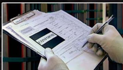
*The results of this careful control, combined with the transferred data in the electrical paper of the single piece that follows the product for the whole manufacturing process, give rise to the conformity and test certificate.*
